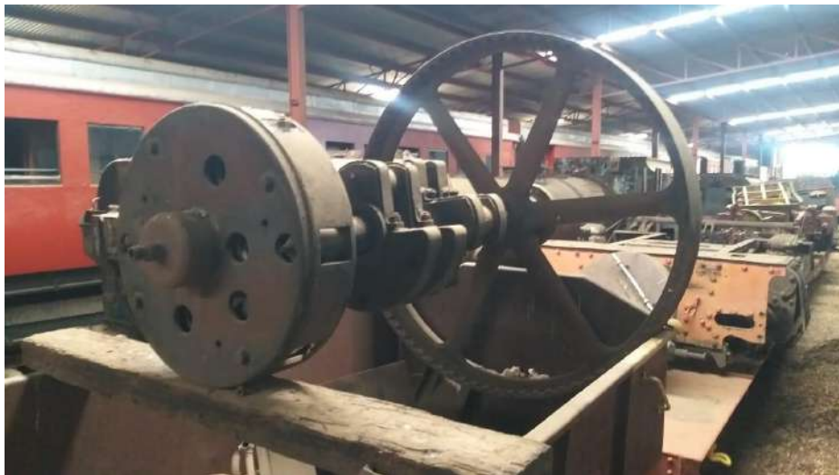
The crankshaft of the Garrett in the "B" wagon.
