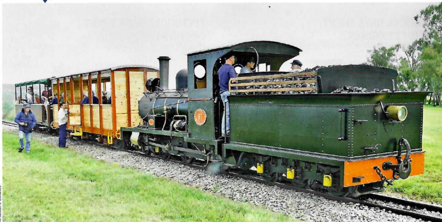
5 Rear view of 4-4-0 n° 97 showing the tender with its bunker extensions.
