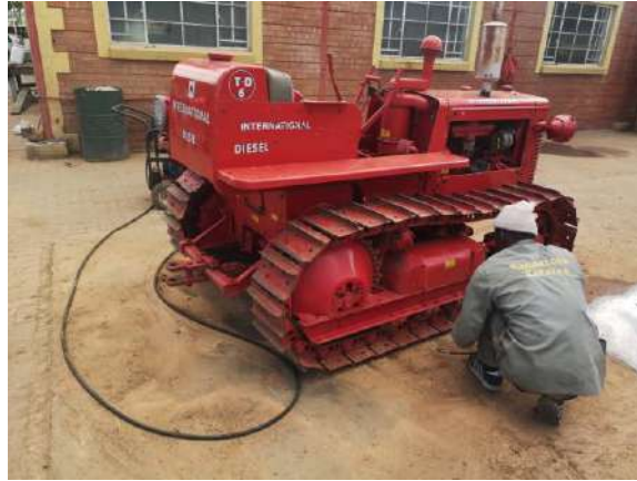
After a good wash the IH TD6 track rollers got a lube from James.
