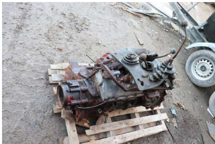
The Cascade type gearbox.
