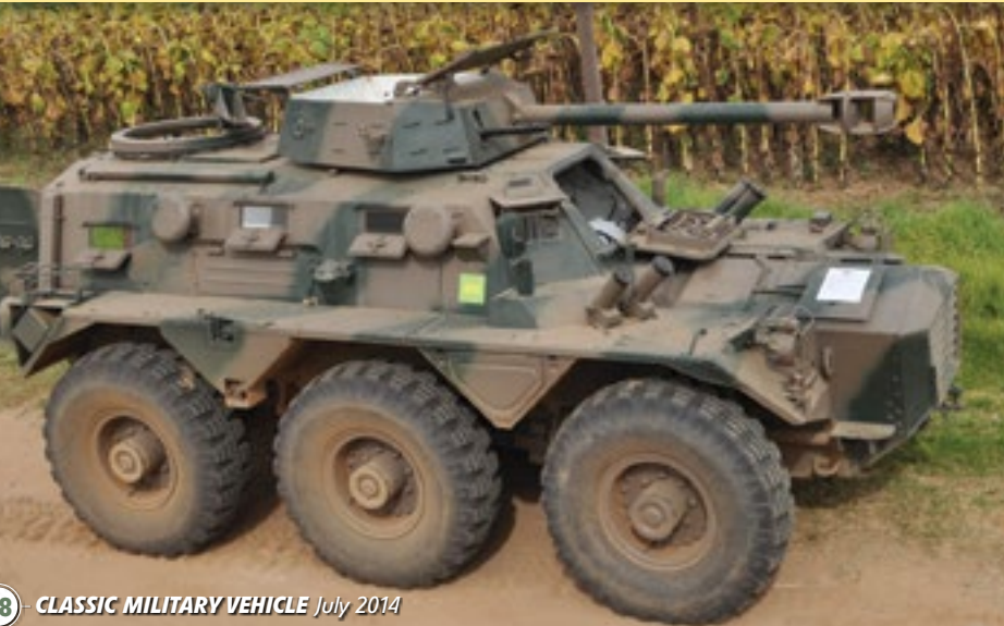
Above: The Eland 60mm mortar originated from the French Panhard but had a 2.5-litre Chevrolet engine and was assembled in South Africa during the Bush War. It formed the mainstay of South African armoured units.
