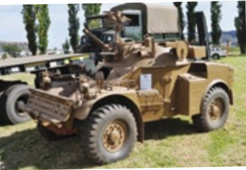
Above: The Eland 60mm mortar originated from the French Panhard but had a 2.5-litre Chevrolet engine and was assembled in South Africa during the Bush War. It formed the mainstay of South African armoured units.
