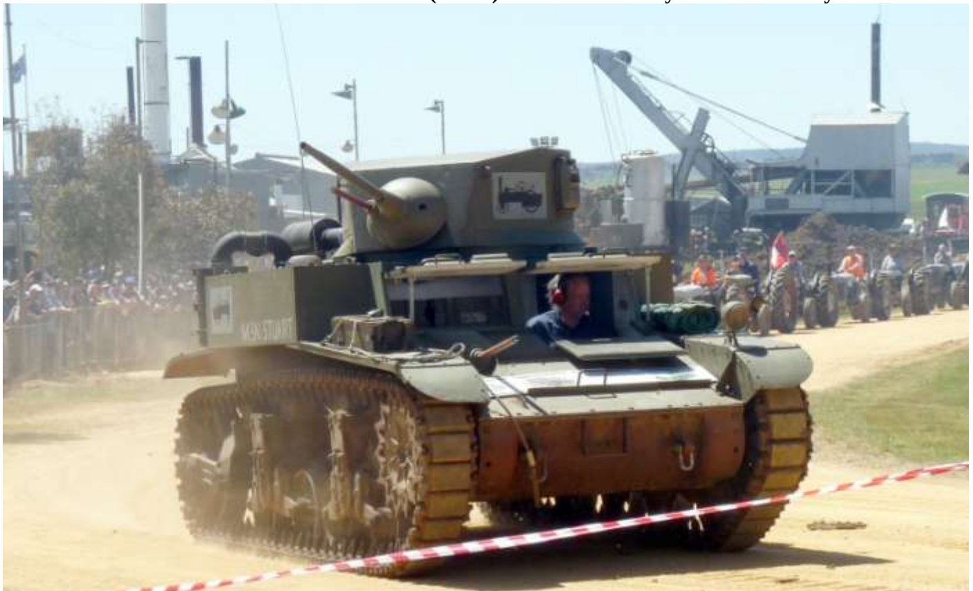
The Stuart does a quick lap around the Arena Parade Ground in November 2012 The same Tank on the Parade Ground on November 2016. The major hull work has been completed and a Rotating Turret has been added and a “ new” set of tracks have been fitted.
