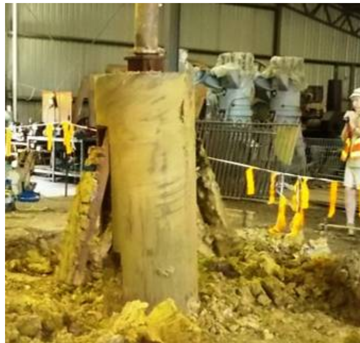
Above and Right The Bellmouthing tool has toothed arms that are forced out by downward pressure on the drive shaft .
