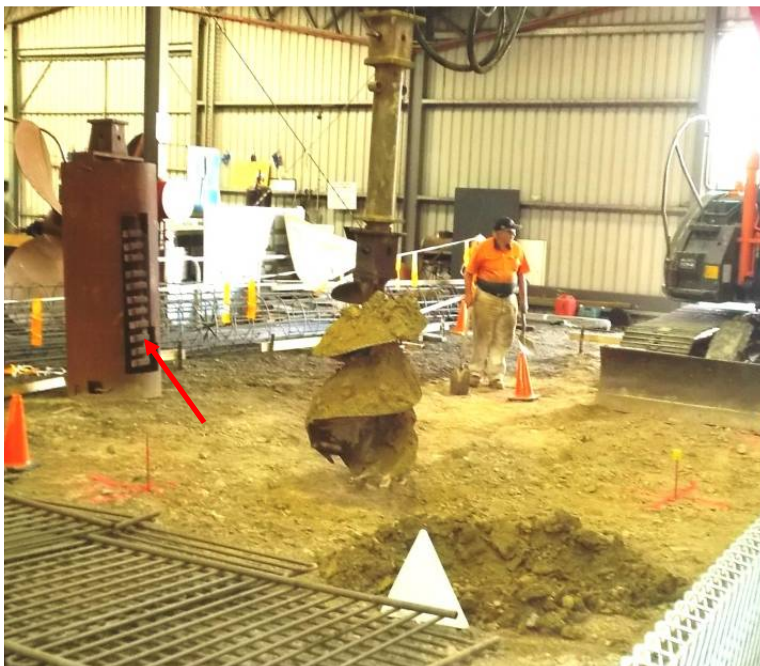
Above and Right The Bellmouthing tool has toothed arms that are forced out by downward pressure on the drive shaft .
