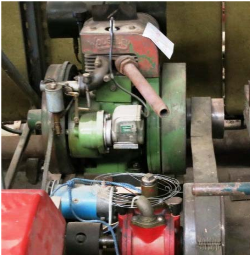
Above A close up view of the Wolseley air cooled 4 stroke single cylinder petrol engine. Don has set it up to represent a typical installation of it's day. Engines of this type could be heard starting up at milking times all over the valley.
