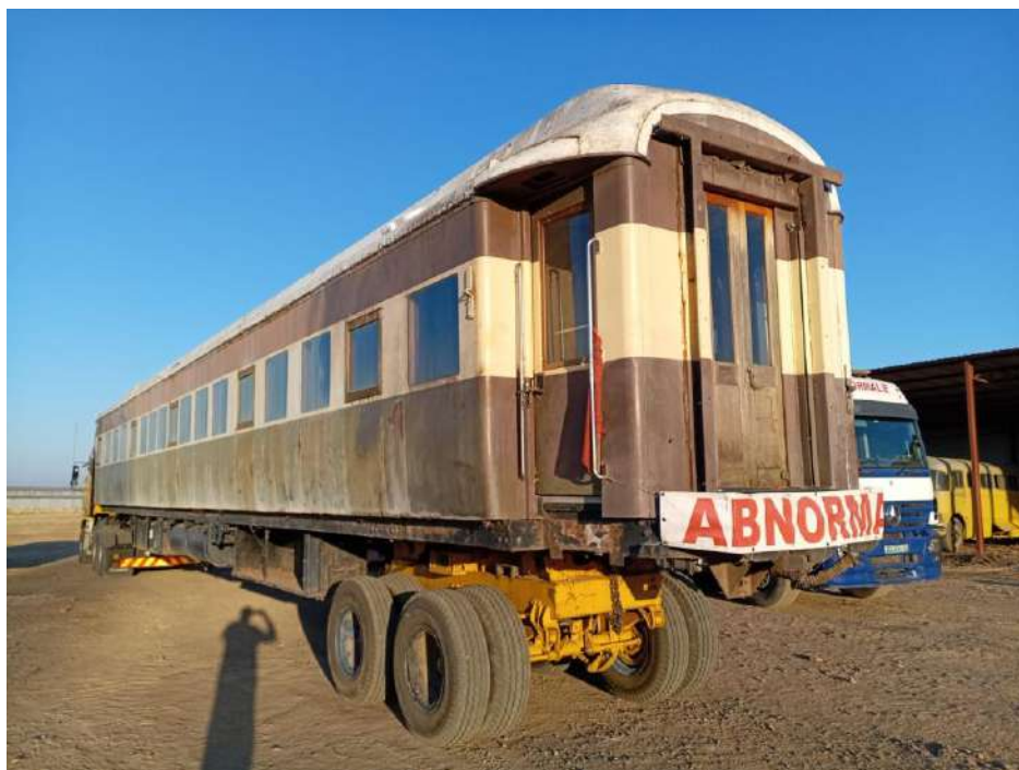
The road dolly in position at the rear of the coach
