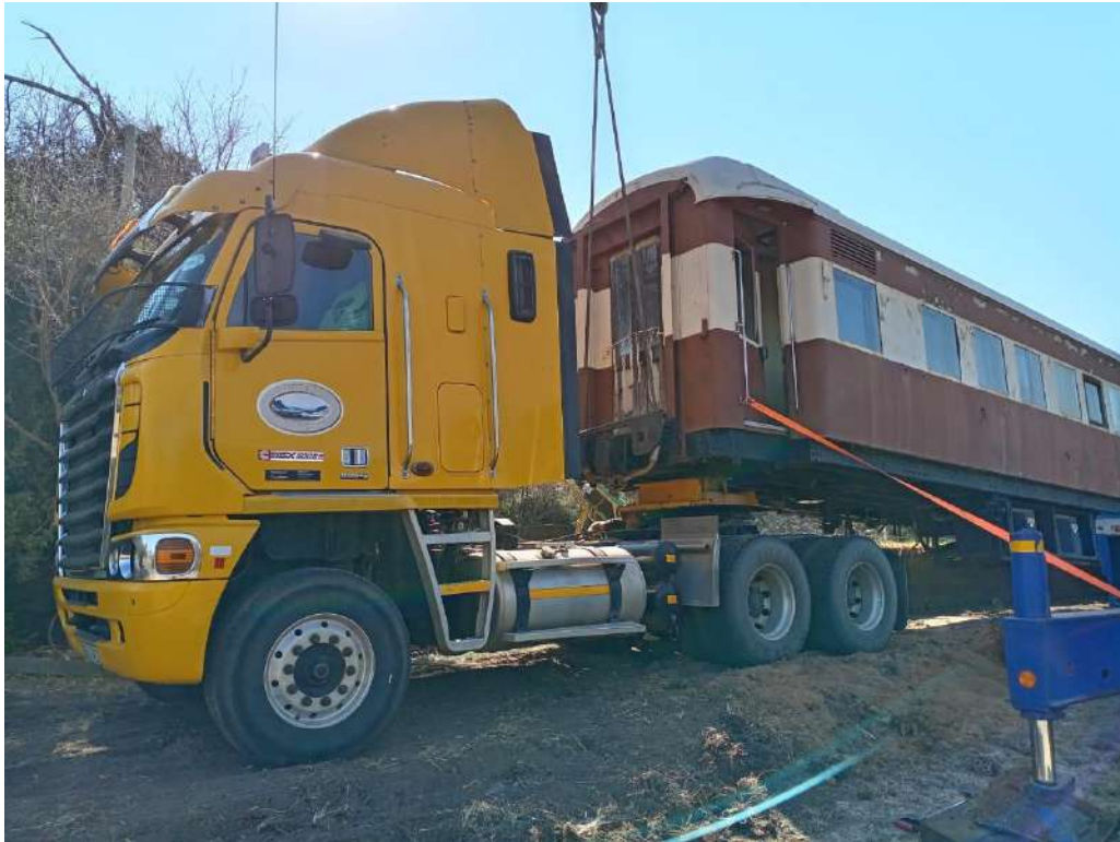
The first coach lifted off their front rail bogie and placed on a special 5 th wheel mounting on the Sandstone truck.
