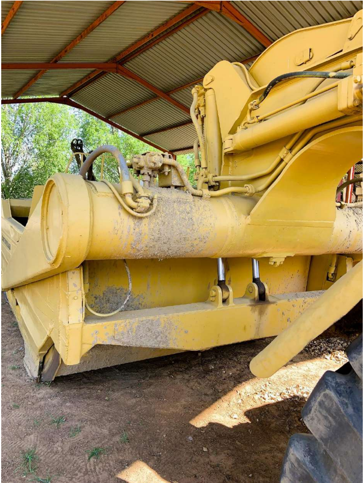
The lower end of the bin cylinders.
