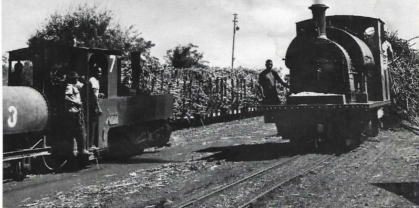
Action at Marromeu! A former German Feldbahn 0-8-0T, built in 1918, meets an English Peckett 0-6-0ST, 31 years its junior. The Peckett, itself a small engine, looks huge in comparison with the Feldbahn — check the size of the men.
