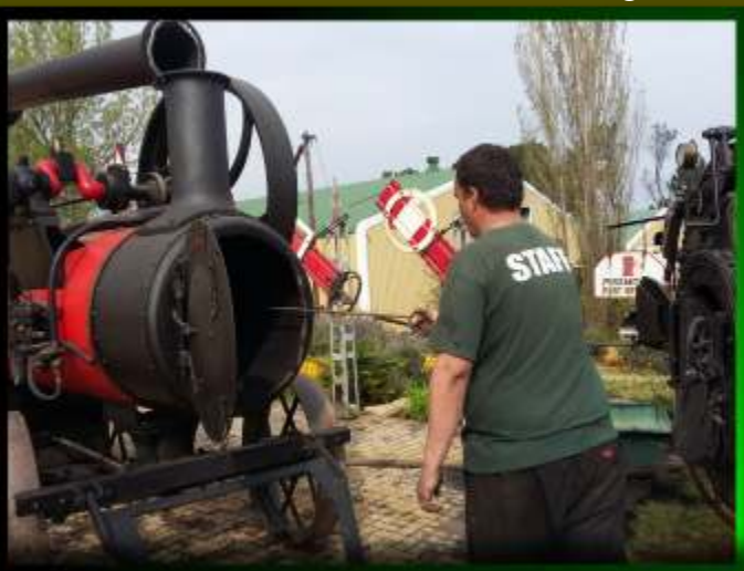
Below left: Tubes cleaned with a special tube cleaner. Below right: The smoke box being wire brushed.
