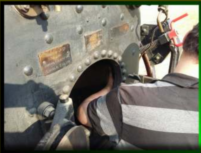
Below right: Cleaning all soot from the tubes with a tube cleaner.
