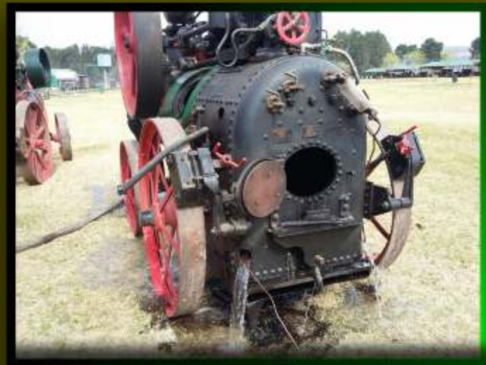
Below right: Cleaning all soot from the tubes with a tube cleaner.
