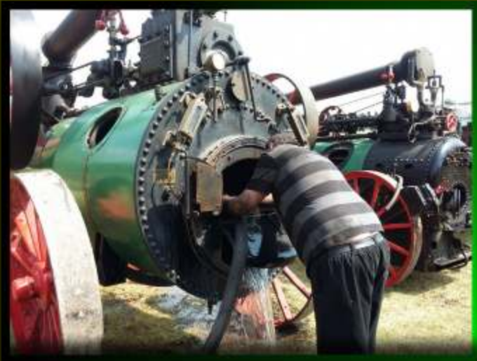
Below: Washout of the Marshall Portable.
