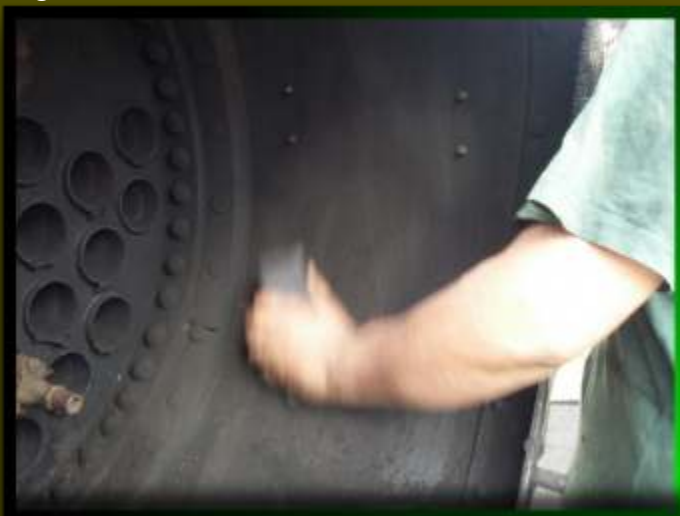
Below left: Tubes cleaned with a special tube cleaner. Below right: The smoke box being wire brushed.
