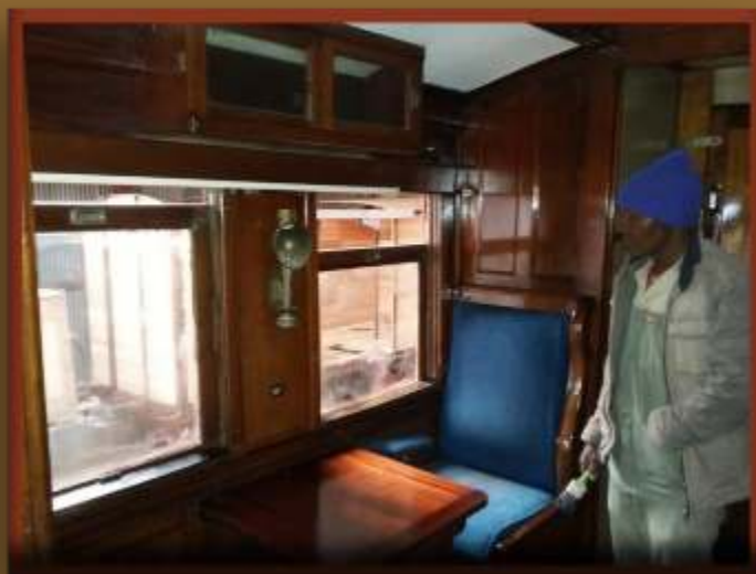
Below right: Brian and Agnus then started and varnished the interior of the Dining coach.
