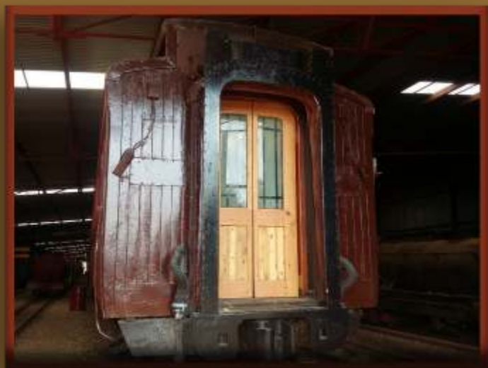
Below: The new origin pine doors fitted.
