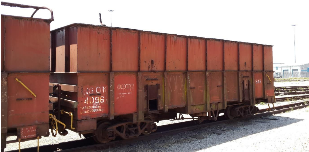
A high sided C3 type, number 4096, modified from an original C1 type stands at Baakens River in Port Elizabeth before being moved to Sandstone. The original lower sides of the C1 can be seen plus the added sliding doors for the discharge of cargo. Photo by David Richardson.
