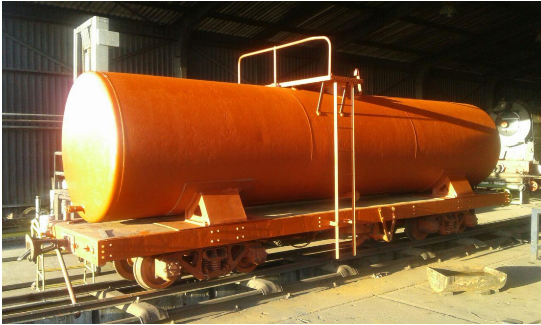
X type tanker number 2197, built in 1952, was restored alongside NGG11 number 52 at Bloemfontein to act as an additional water supply for the locomotive. Photo by Lukas Nel.
