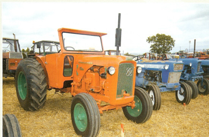
Largely unknown in the Northern Hemisphere, the Australian Chamberlain 9G 'Champion' is something of a legend in its home country after one took part in a trans-continental car race in the fifties! Not as crazy as it sounds, as the 9G was a fast road tractor capable of around 50km/h while also able to tackle almost any terrain. A rare sight outside Australia, it was a fitting tribute to such a unique event to have such a special machine taking part.
