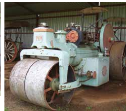
Aveling No.5396, unusually fitted with a large belly tank and one of a trio of similar rollers – designated as a 'Special Road Roller' – and the first of a trio of identical 12 ton rollers supplied to 'Crown Agents for the Colonies' on 25th November 1903, destined for Pretoria in South Africa!
