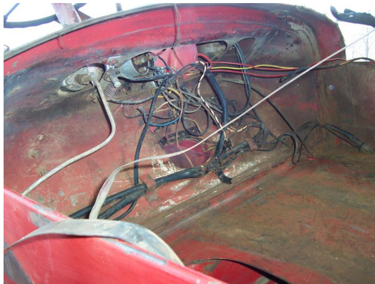
Several generations of wiring, mostly nonfunctional to be sorted & replaced, after the cavity has been cleaned & decades of filth removed.
