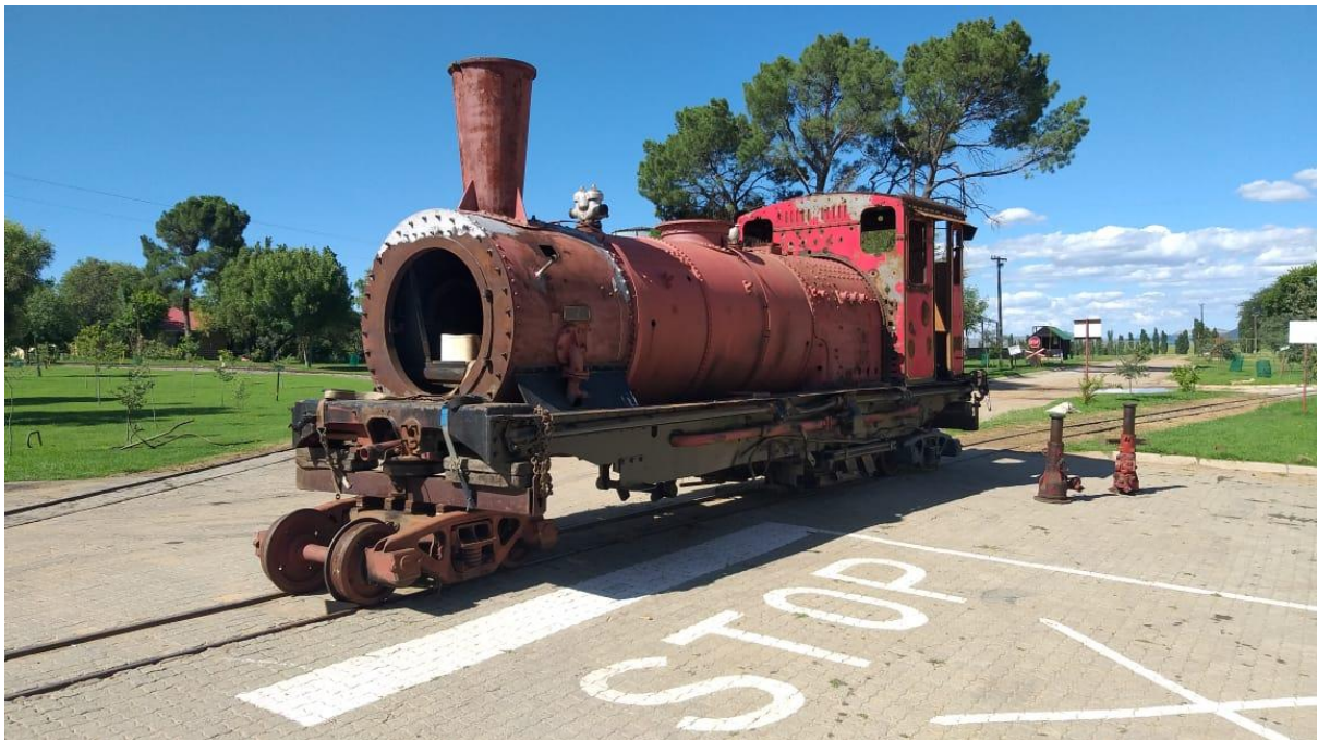
Split from its engine units, number 155 awaits loading at Sandstone for its journey to the boiler repair shop.
