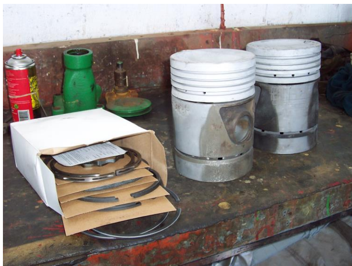
The pistons repaired with new rings awaiting assembly and the stripped water pump in background.
