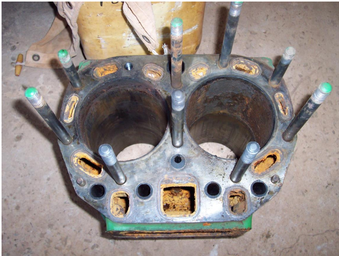
The cylinder bores, rusted but salvageable.
