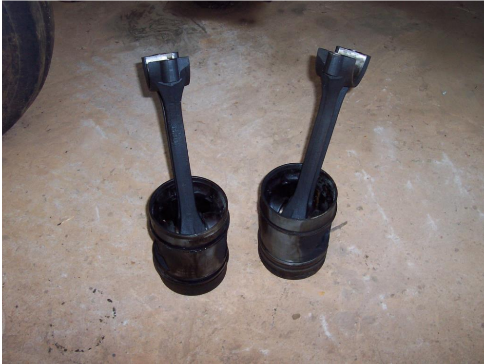
Initially the forcefully removed pistons looked good – but closer examination showed broken ring lands disguised by hard carbon deposits.
