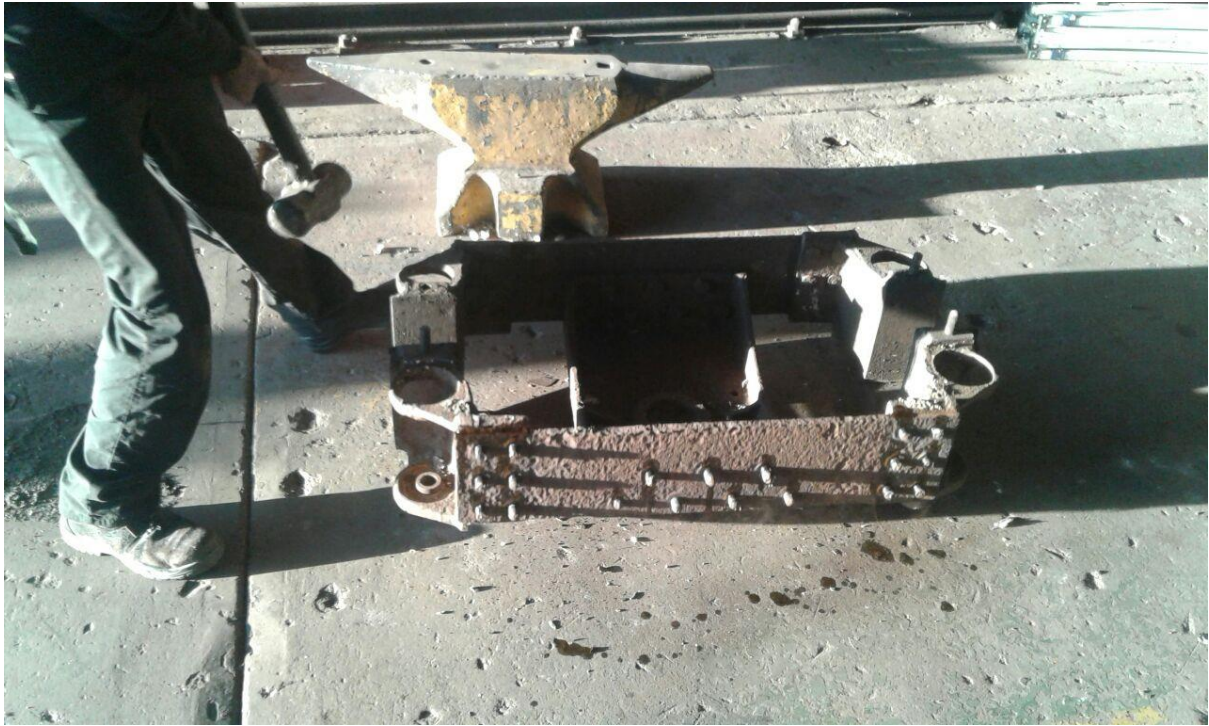
The rusted bissel frame
