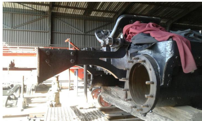
Another view of the buffer beam.
