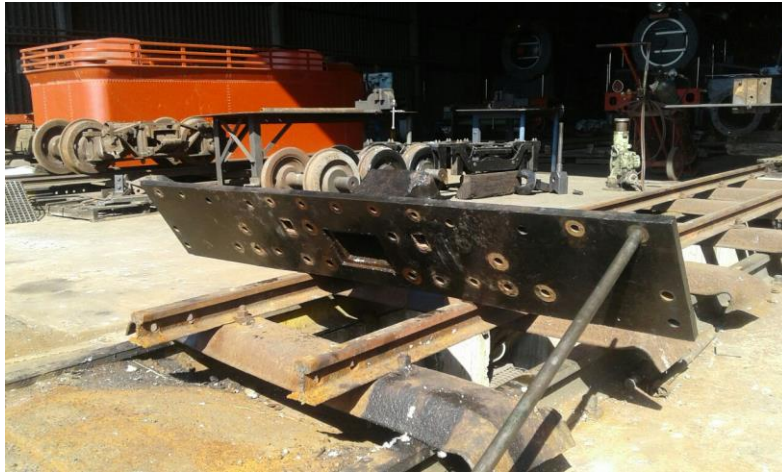
The buffer beam after being re-aligned.
