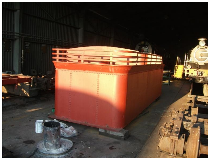
The new tender tank.
