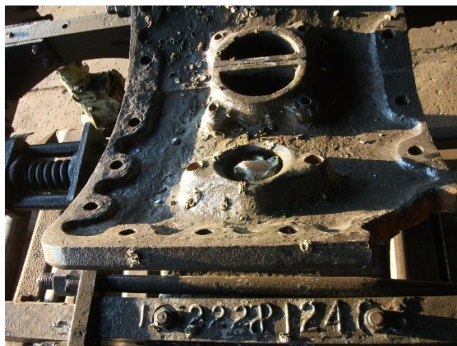
The NG10 boiler saddle casting.
