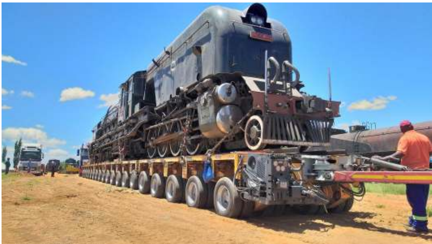
The massive size of the multi axle trailer and its GMA/M load is evident in this picture. Picture Sandstone Heritage Trust.
