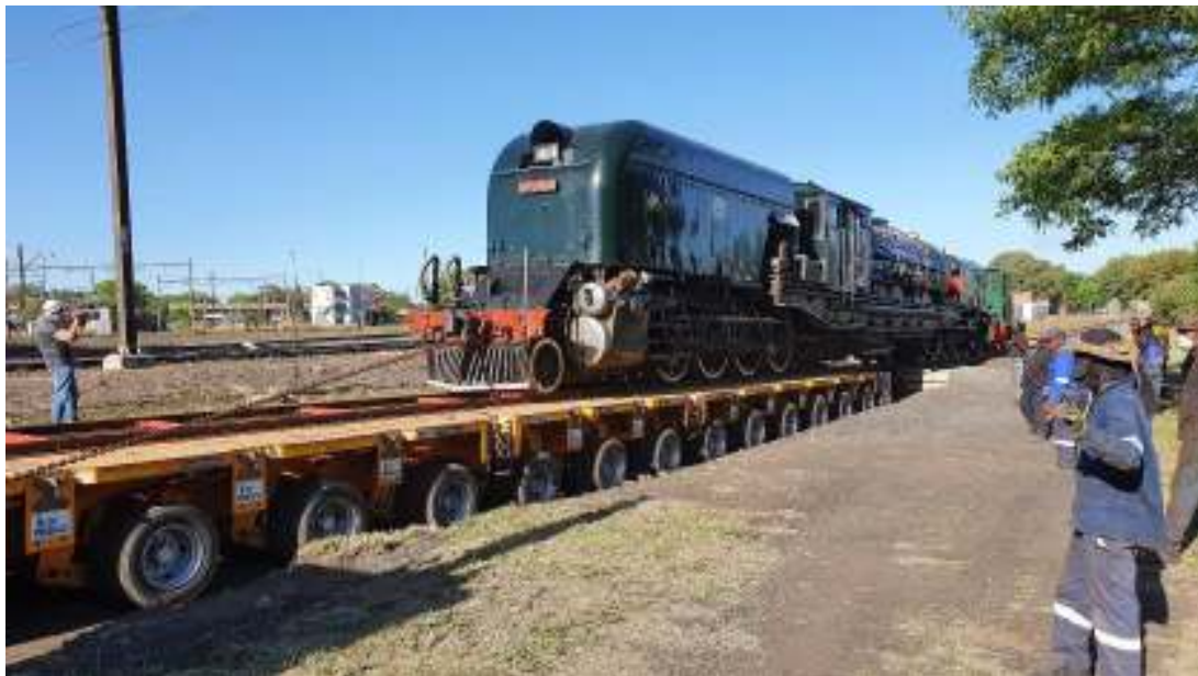
GMA/M 4079, "Lyndie Lou" is winched on to the multi axle trailer. At 154000kg, just too much for the mighty Hunslet! Picture by Sandstone Heritage Trust.
