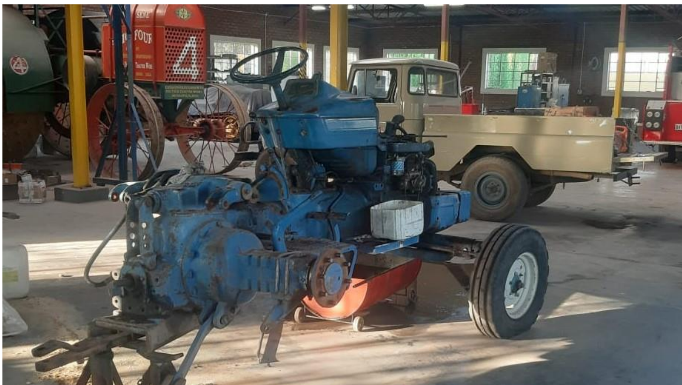
The Ford 5000 stripped down in the Sandstone workshop
