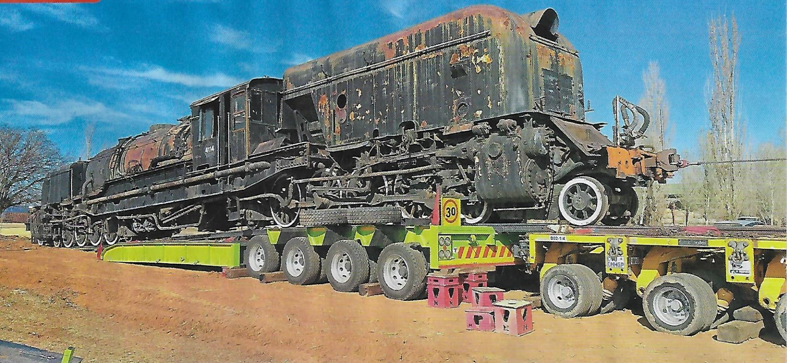
Glasgow-built articulated GMAM Garratt 4-8-2+2-8-4 No. 4114 of 1957 on its way to permanent safety at Sandstone Estates. GERT JUBILEUS
