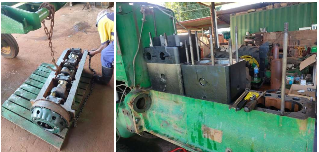
The crankcase is ready to be mounted to the chassis and on the right, in situ, you can clearly see two of the separate cylinder blocks.
