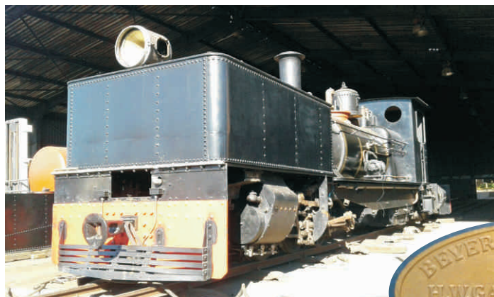
Above: the new tank in place Below: together with the sanders and cylinder cock equipment in place behind the buffer beam.
