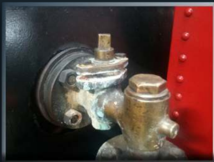
Below: The signs of leaking is evident in all the pictures, the white is all leaking joints and glands.
