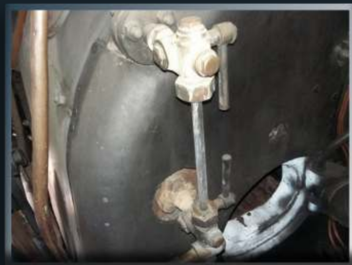
Below: The signs of leaking is evident in all the pictures, the white is all leaking joints and glands.
