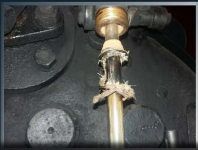
Below: The signs of leaking is evident in all the pictures, the white is all leaking joints and glands.
