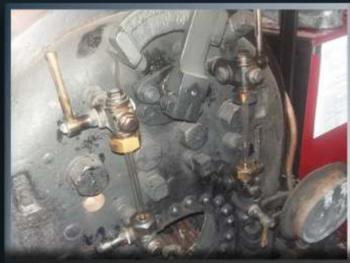
Below: The signs of leaking is evident in all the pictures, the white is all leaking joints and glands.
