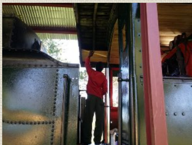
Below right: Brian busy painting the chimney and smoke box with the same graphite look paint of the bogeys.
