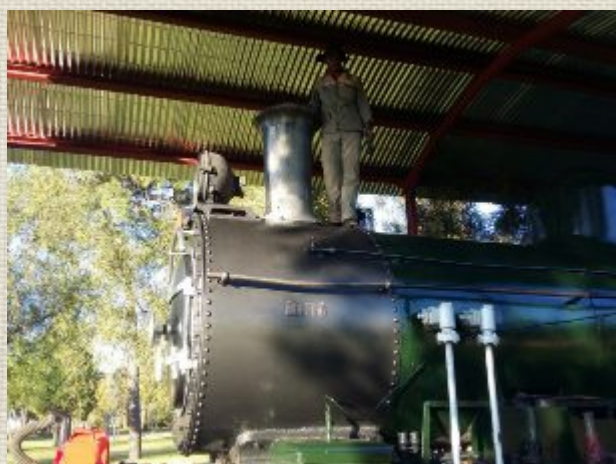
Below right: Brian busy painting the chimney and smoke box with the same graphite look paint of the bogeys.
