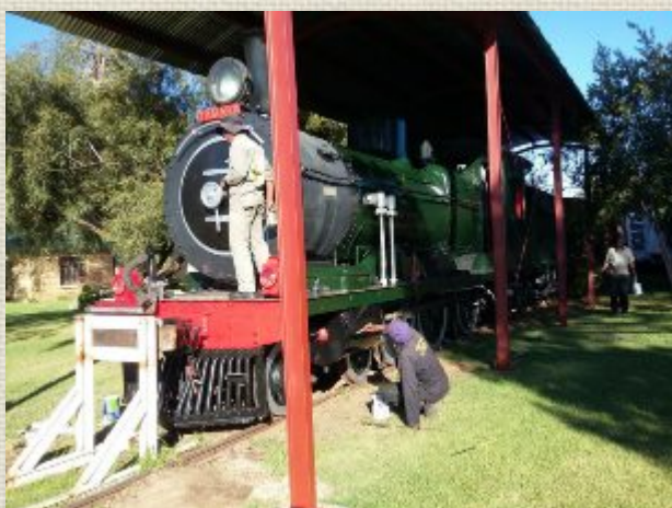
Below right: Brian busy painting the chimney and smoke box with the same graphite look paint of the bogeys.
