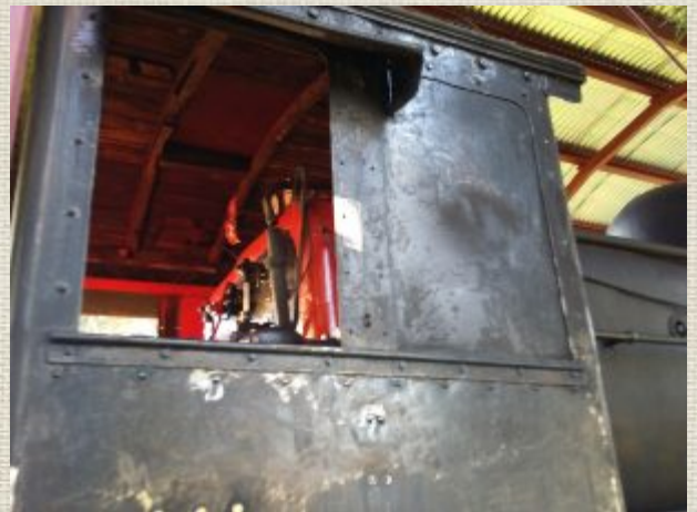
Below: The cab sides after sanding it with the flapper disks..
