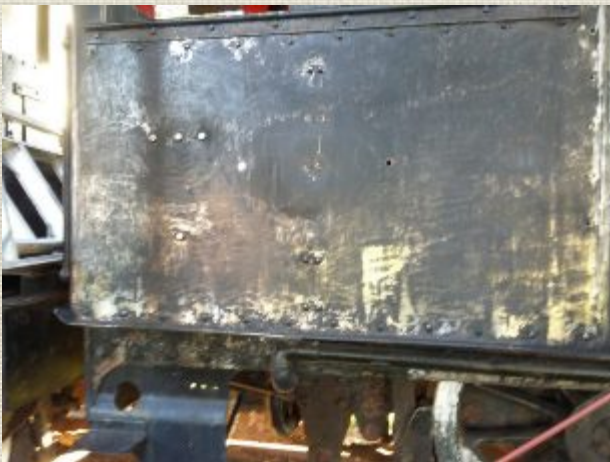
Below: The cab sides after sanding it with the flapper disks..
