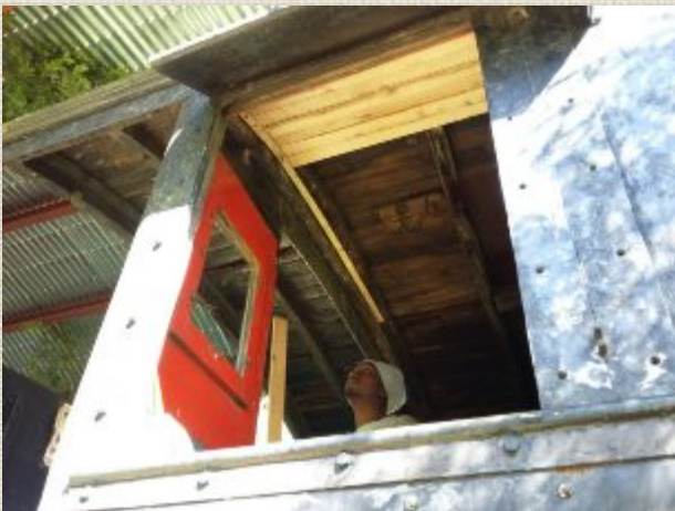
Below: The new wooden roof being fitted.
