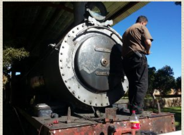
Below : Cleaning the smoke box head plate.
