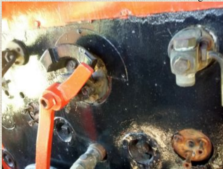
Below: Gauge column corks being fitted.
