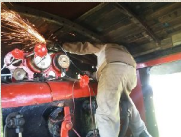
Below: Joseph preparing to fit the new wood roof of the Class 6C
