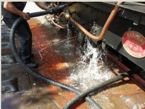
Below: Mud and scale being washed out.
