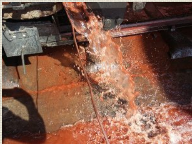
Below: Mud and scale being washed out.
