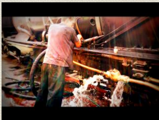
Finally we cleaned the tubes and ensured that no one is blocked with cinders.
