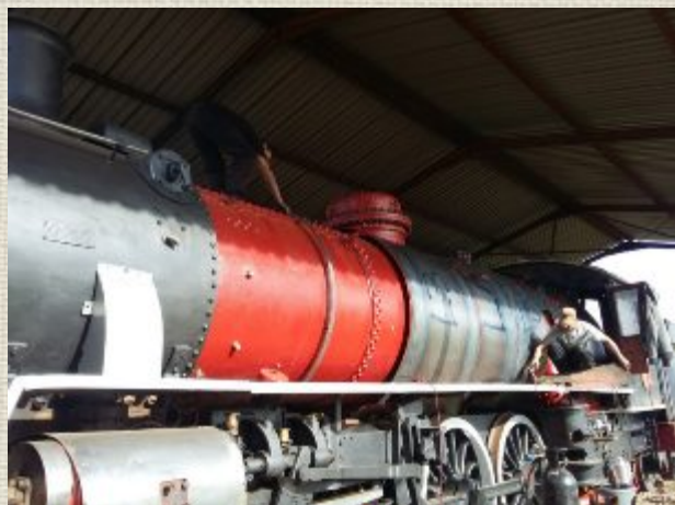
Below left: Brian did the most of the paint work on the Class 10 CR while Petrus, Johannes and Joseph Scraped of all the old paint.
