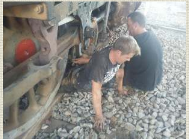
Below left: A set of old gauge column corks were fitted. Below right: Thinus busy fitting the cylinder corks back.
