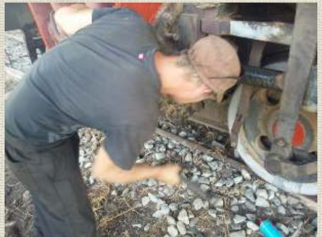
Below right: Connecting the braking gears and finally the last brake blocks.
