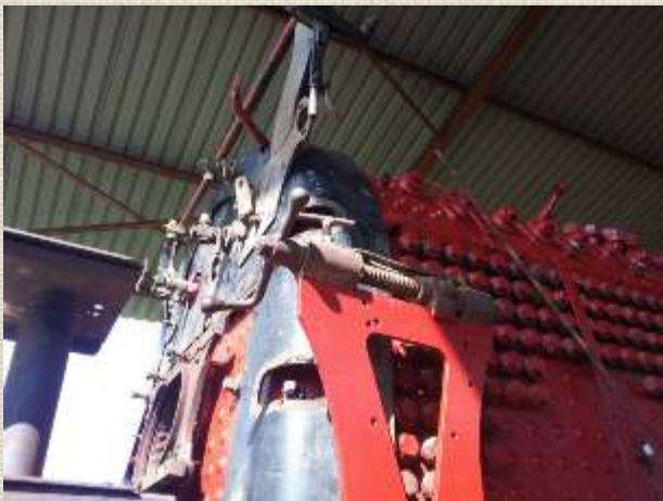
Below right: Connecting the braking gears and finally the last brake blocks.
