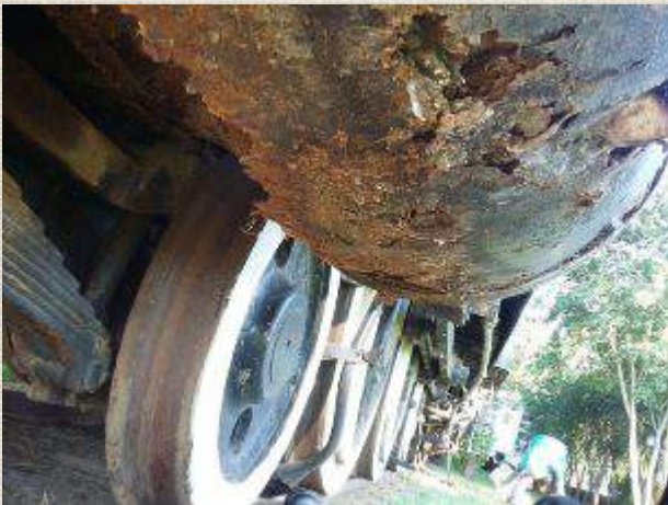
The locomotive now will be sanded down before we will start with painting her.
