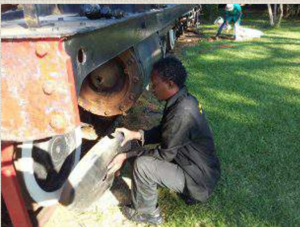
The locomotive now will be sanded down before we will start with painting her.
