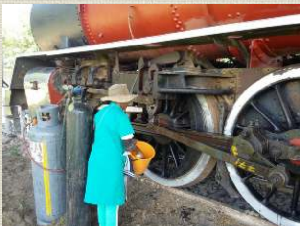
Below: The motion was cleaned and Brian painted it with a special graphite mix.
