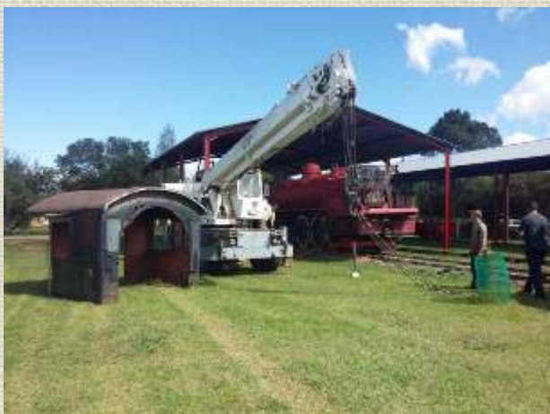
The Class 10CR locomotive was out and Henry operated the crane to fit back the cab of the locomotive.
