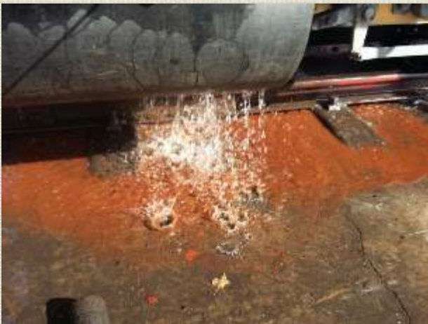
Below left: Washing out from the smoke box end towards the foundation ring where we could Remove all the scale and sludge from the boiler.
