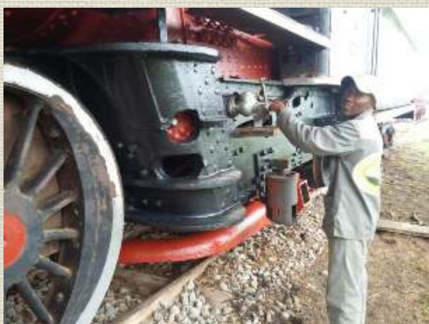
Cecilia first cleaned off all oil and grease with diesel and cloth and then washed the wheels and motion With degreasing fluid to enable Brian to paint the wheels and rods.
