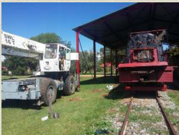
The Class 10CR locomotive was out and Henry operated the crane to fit back the cab of the locomotive.
