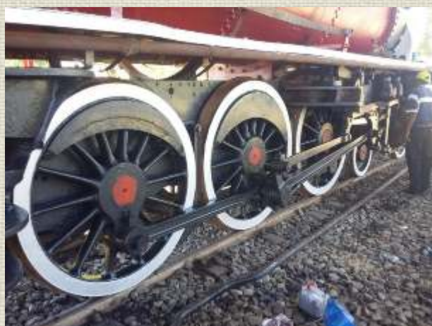
Below: The motion was cleaned and Brian painted it with a special graphite mix.
