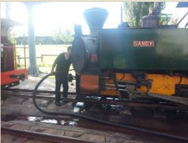
Below left: Washing out from the smoke box end towards the foundation ring where we could Remove all the scale and sludge from the boiler.
