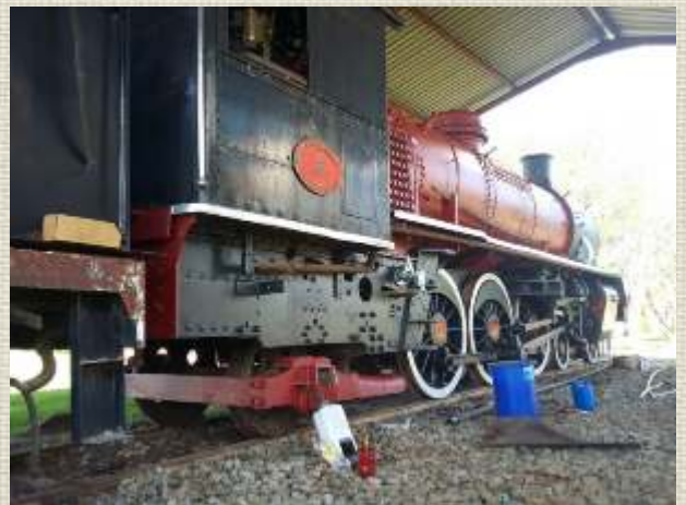
The steel plates for the new cladding was delivered on Thursday and Thinus and Wouter started with The metal work and making up of the new cladding for the Class 10CR.
