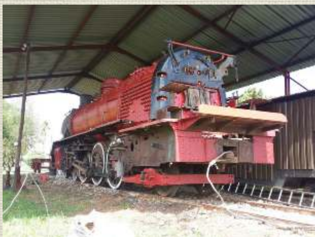
The Class 10CR locomotive was out and Henry operated the crane to fit back the cab of the locomotive.
