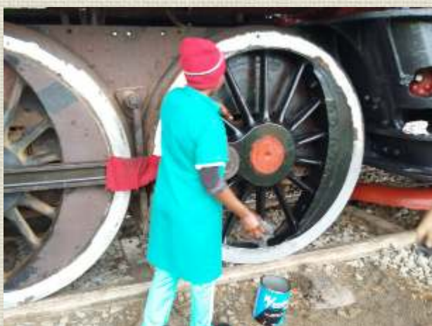
Cecilia first cleaned off all oil and grease with diesel and cloth and then washed the wheels and motion With degreasing fluid to enable Brian to paint the wheels and rods.
