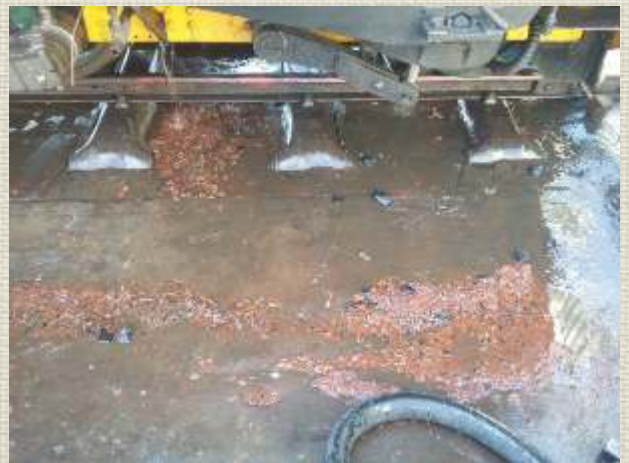
Below left: Washing out from the smoke box end towards the foundation ring where we could Remove all the scale and sludge from the boiler.
