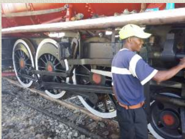
Below: The motion was cleaned and Brian painted it with a special graphite mix.
