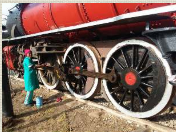
Cecilia first cleaned off all oil and grease with diesel and cloth and then washed the wheels and motion With degreasing fluid to enable Brian to paint the wheels and rods.
