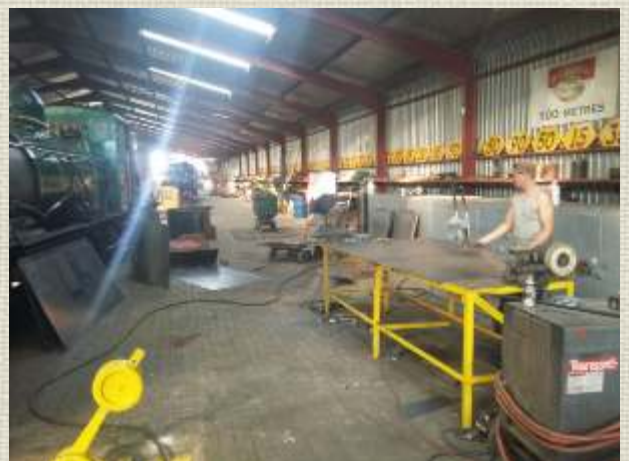
The steel plates for the new cladding was delivered on Thursday and Thinus and Wouter started with The metal work and making up of the new cladding for the Class 10CR.
