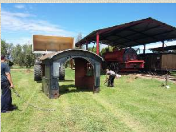
The Class 10CR locomotive was out and Henry operated the crane to fit back the cab of the locomotive.
