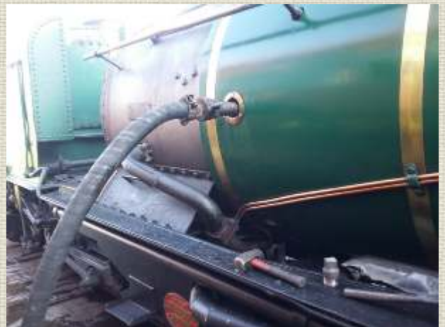
Below: Dissolved scale was washed out of the boiler.
