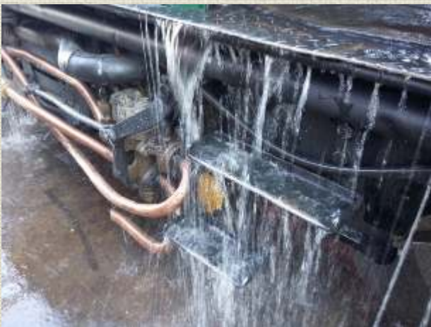
Below: Dissolved scale was washed out of the boiler.
