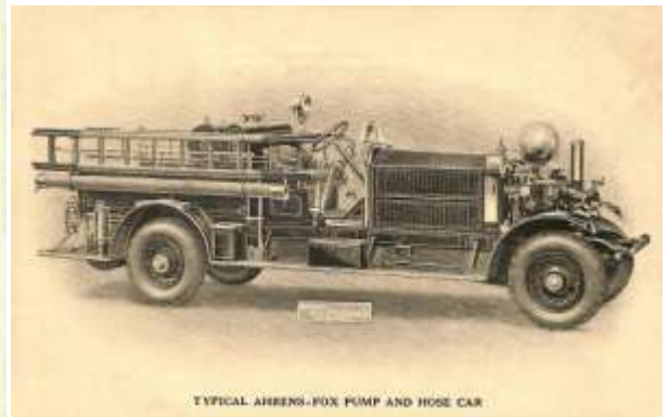
1914 saw the first Ahrens-Fox fire engine with the characteristic front mounted pumps
