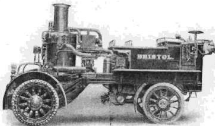
ENGINE ARRANGED FOR CONVEYANCE SUSPENDED ON TRUNNIONS ON TWO-WHEEL CARriage FROM WHICH IT IS LOWERED TO THE GROUND FOR WORKING. CARriage IS DESIGNED FOR HAND-DRAUGHT, BUT CAN BE FITTED WITH SHAFTS FOR HORSE.
