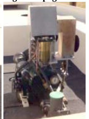
This boat was unusual in that it uses a Sterling Cycle engine. It is certainly a neat layout, and a rare exhibit.
