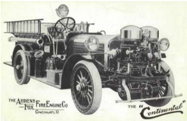
1914 saw the first Ahrens-Fox fire engine with the characteristic front mounted pumps
