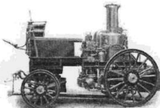
ARRANGEMENT OF ENGINE AT FRONT OF BOILER TO MEET SPECIAL REQUIREMENTS.
