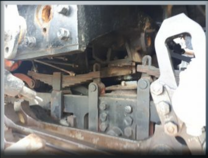
Below right: The second bogie was moved in under the boiler to support the fire box end.
