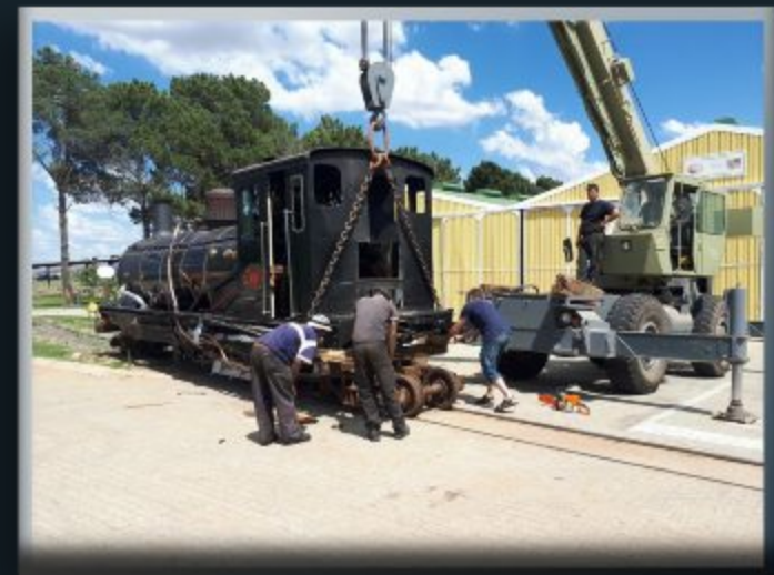
Below right: The second bogie was moved in under the boiler to support the fire box end.
