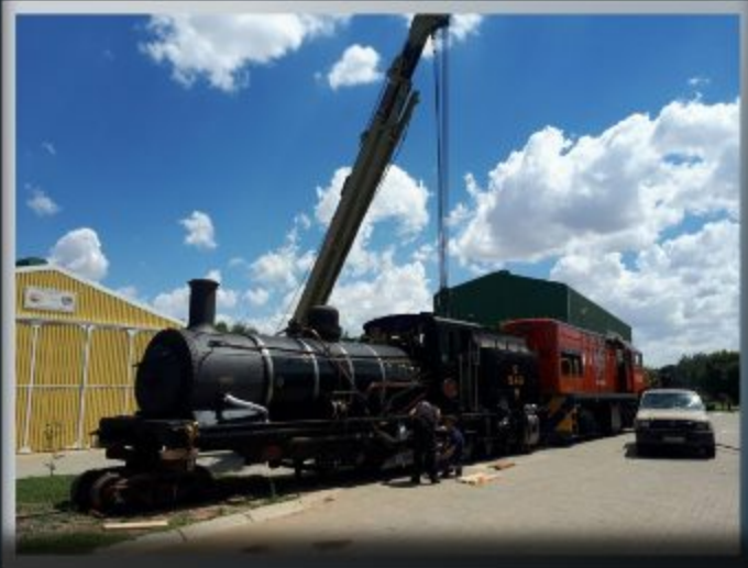
Below left: The crane gently lifted the boiler and the rear unit was pulled out.
