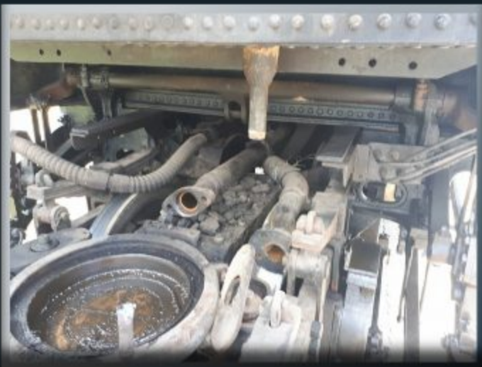
Below right: The second bogie was moved in under the boiler to support the fire box end.
