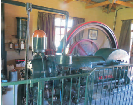
Right, the valve gear responsible for the rhythmic “clackity clack” sound which attracts the visitors when the engine is running
