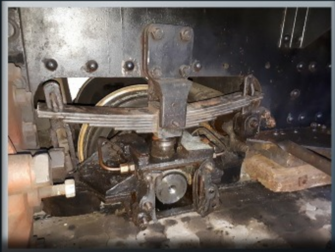
Above left: A spring was fitted on the front pony wheel.
