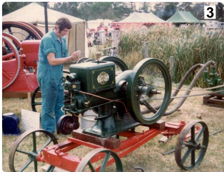
Above International 6 hp petrol engine built in USA in 1922 and owned by Ross Foster set up to pump on the bank of the lake in the background.
