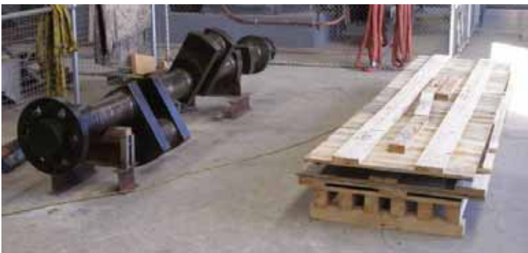
Above A shipping crate flat pack of specially treated timber . Once the crank is screwed to the base the sides and lid will be attached.
