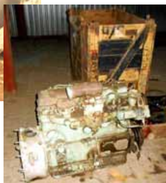
Below The pressure was really on these Armour Museum volunteers to make an emergency over night engine change on this Ferret Scout car . Enthusiasts were invited to visit the Sandstone workshops to inspect the proceedings . Although busy the mechanics still had time to tell me the original engine was malfunctioning due to the oil and petrol being mixed up .
