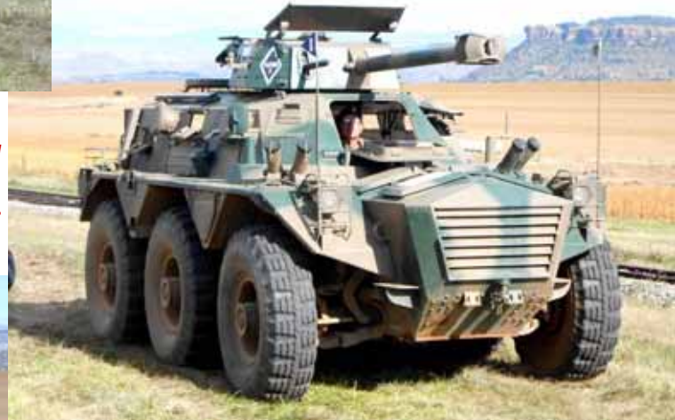
Right Saracen Personnel Carrier of British origin using Rolls Royce straight 8 petrol engine but South African modified with larger wheels suit local conditions, 1950s to 1970s . These were superseded by the South African made Buffel mine proofed troop carrier shown Below
