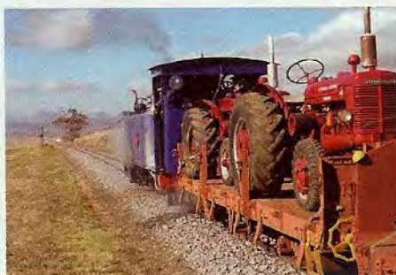
Ex SAR 1913 NG14 1344 Kerr Stuart 4-6-2 side tank, one of seven built to work on the Alfred County Railway from Port Shepstone to Harding line. A full rebuild was given to this 30 ton locomotive in the mid 2000s and it took its turn on the tractor train here.
