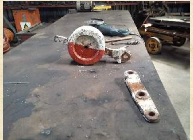
Below: Hoekfontein South mainline points bended. Wouter removed it and made it straight again.
