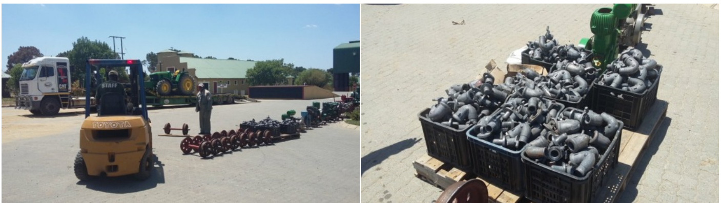
Below right: Brand new vacuum pipe couplers and goosenecks for our wagon restorations.
