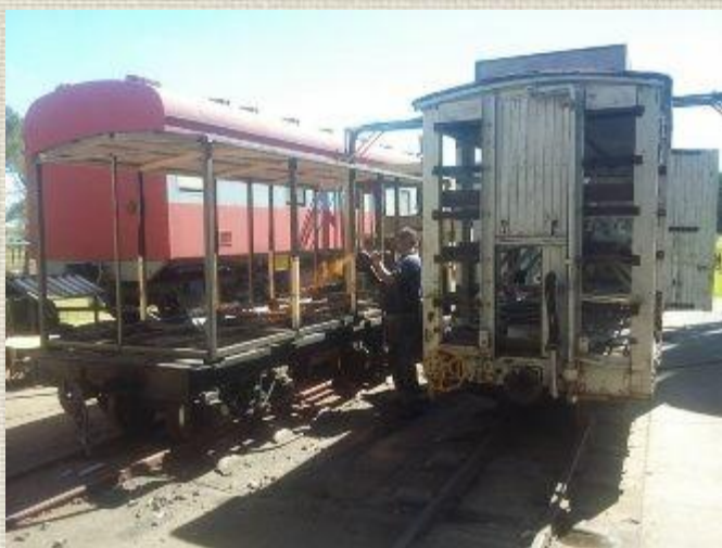
Below left: Final grinding of edges before the wagon was shunted to the new Wagon Shed For the woodwork to commence.
