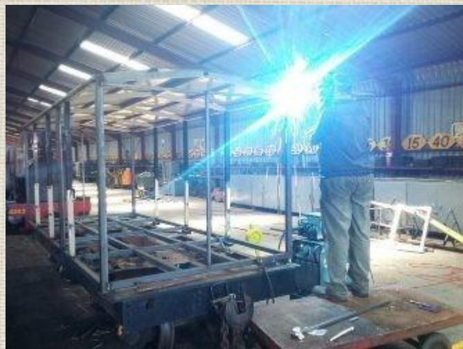
Below left: Final grinding of edges before the wagon was shunted to the new Wagon Shed For the woodwork to commence.
