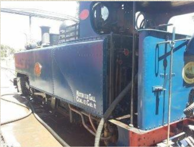
Below: Washout from the smoke box side.
