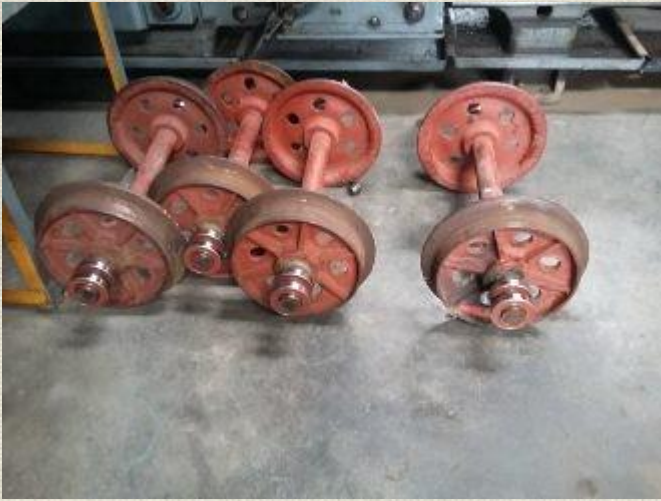
Below left: Axle boxes fitted back and wheels are ready to be fitted under the wagons.
