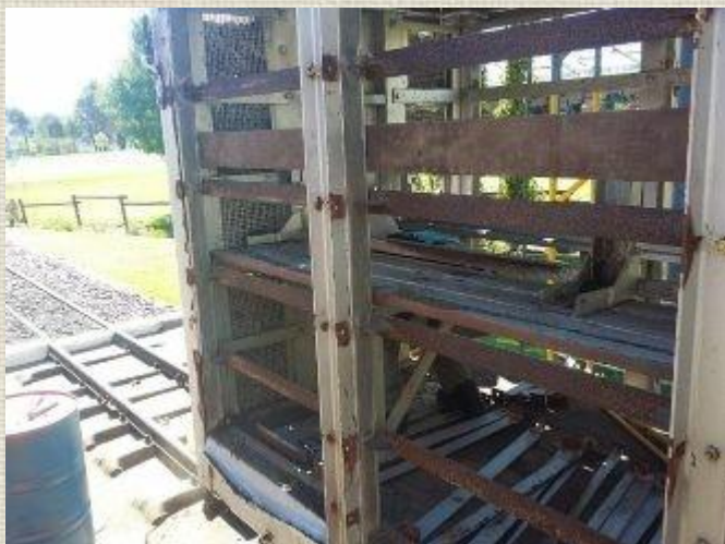
Below right: More planks that needs replacement.
