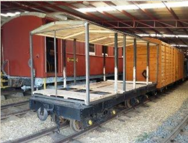
Below: The wood for the floors and Joseph started to mount it to the steel frame.
