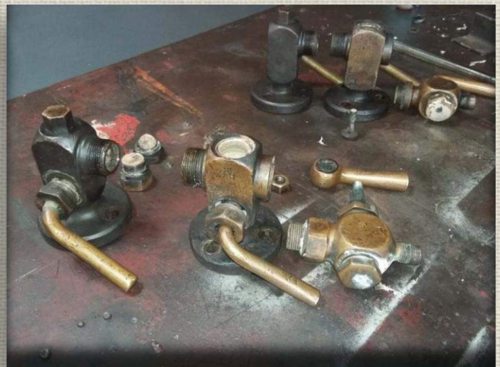
Below: Left and right side steam, water And test corks ready to be cleaned in Diesel over the weekend
