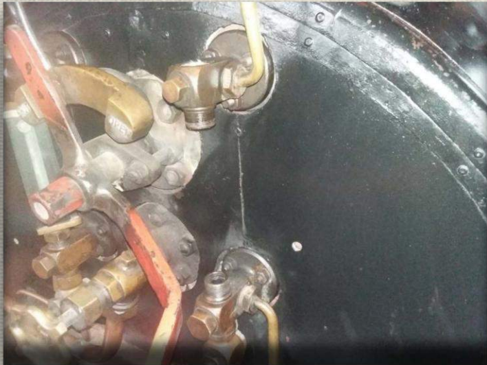
Below left: Gauge glasses removed
