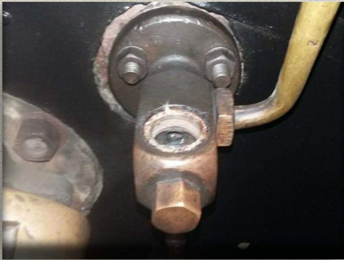
Below left: Gauge glasses removed
