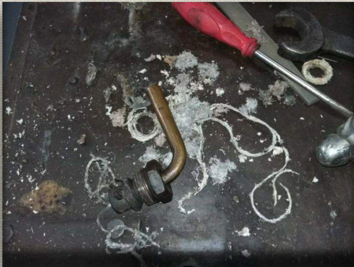
Below: Test cork being stripped and asbestos removed.
