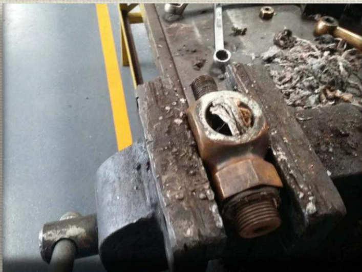
Below left: Some more asbestos removed And the pile of old hardened asbestos Evident in the right side of the photo
