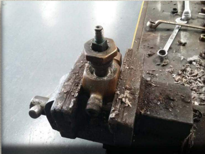
Below: Test cork being stripped and asbestos removed.
