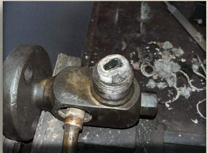
Below: Test cork being stripped and asbestos removed.
