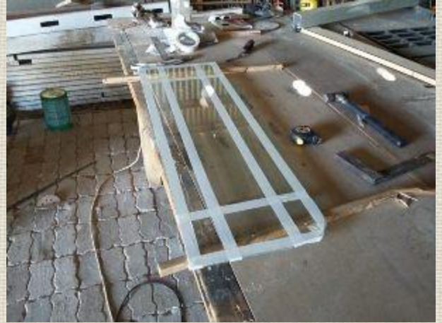
Below: The door glass prepared to be sandblasted.
