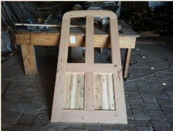
Below: New wooden frames for the larger windows of the Dining Car.
