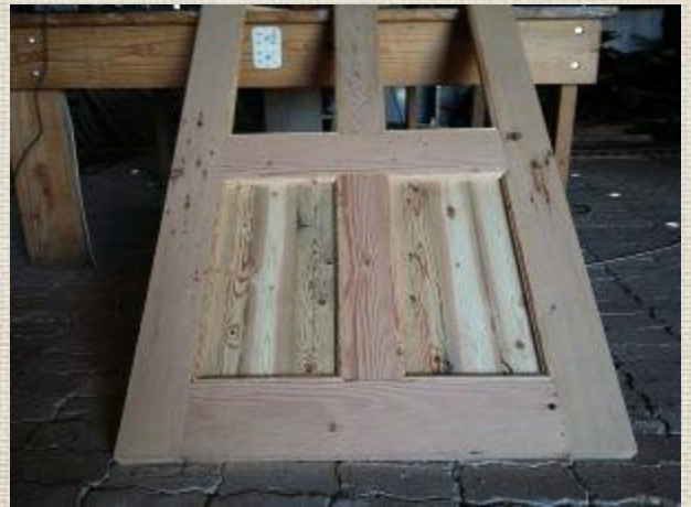
Below: New wooden frames for the larger windows of the Dining Car.
