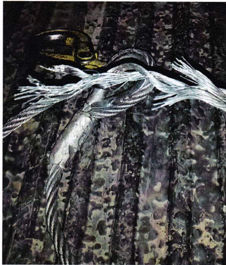
Figure 9: Failed tow cable
