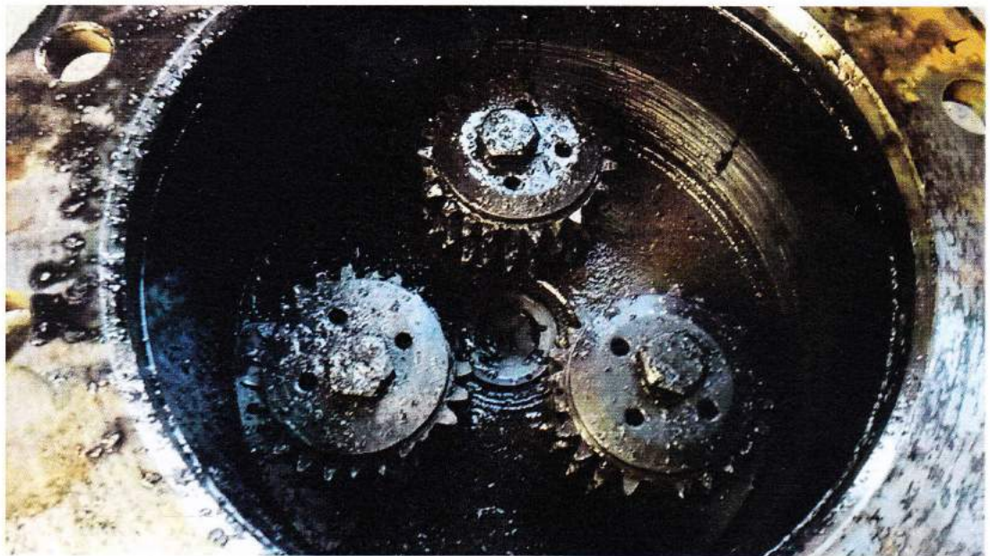
Figure 10: Visual inspection of seized tractor hub
