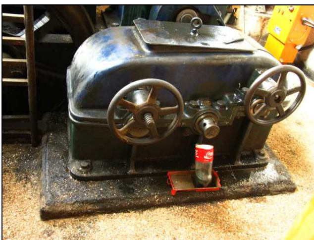
P12 - The idler shaft bearing continued to leak and a simple catch bottle was set up to capture the oil and chuck it back in through the top hatch. The bearing is about 0.5 mm oversize, letting the gear oil sneak through. It isn't a serious problem and it will be re-lined again once the 15CA project is completed. (Note the fresh sawdust on the floor.)
