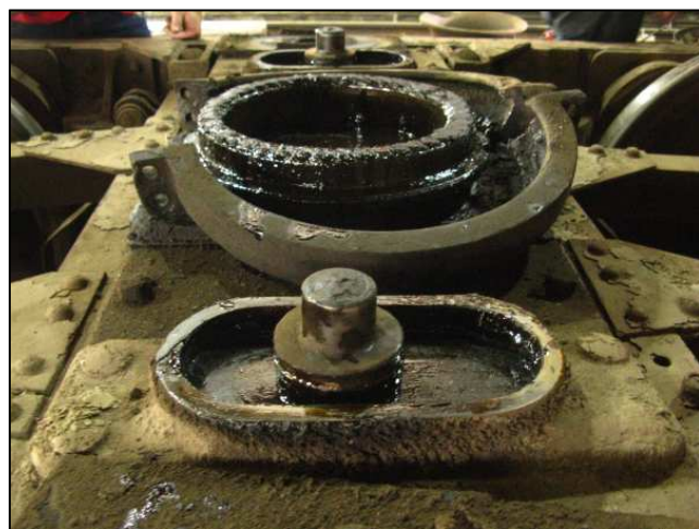
P22 - These old bogies have sliding pads on the shoulders of their bolster beams, and they need cleaning and lubrication. The collars around the bolster pin are nasty to uncouple at arm's length when starting the job
