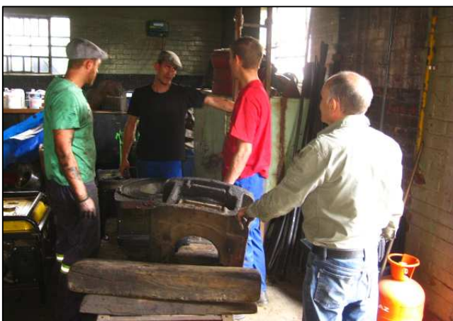
P09 - The axle boxes will be going to Valard Bearings to have their liners melted out and new white metal liners and thrust bearings cast. Valard Bearings do bearing work for us at no charge, and for which we are quite grateful.
