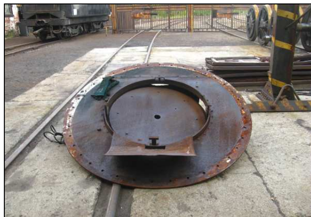
P20 - The rear of the smokebox plate, complete with cinder shield. The similar front plate that Hannes had been grinding down was for the 15CA show-boat project, not for this 15F 3052 locomotive, as I had earlier reported in error.
