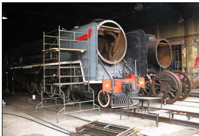
P14 - Sporting new cast wing plates, Sandstone's 15F 3052 has since had the boiler tubes all beaded over at the firebox end ready for the coded welding. Most of the boiler fixtures have since been reinstalled for the coming steam test, but many needed to have wasted steel studs replaced.
