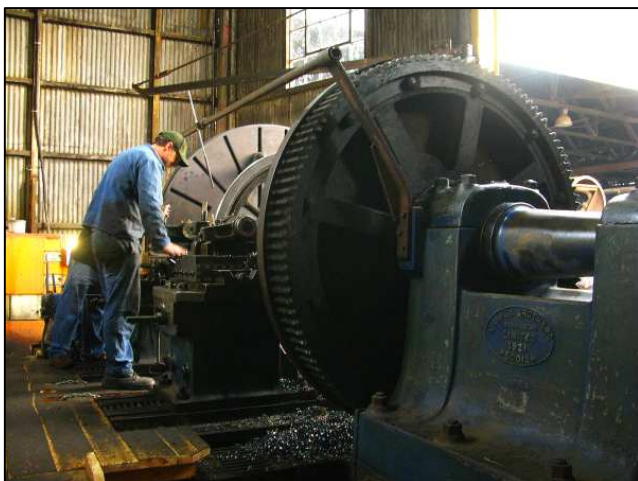
P13 - The big lathe picked up a bit of a chatter as it did during last week's session. The vibration from one side can feed into the other. The fault turned out to be simple – the tool tower racking bolts weren't tight enough. They need to be checked and tightened regularly. Lesson learned.
