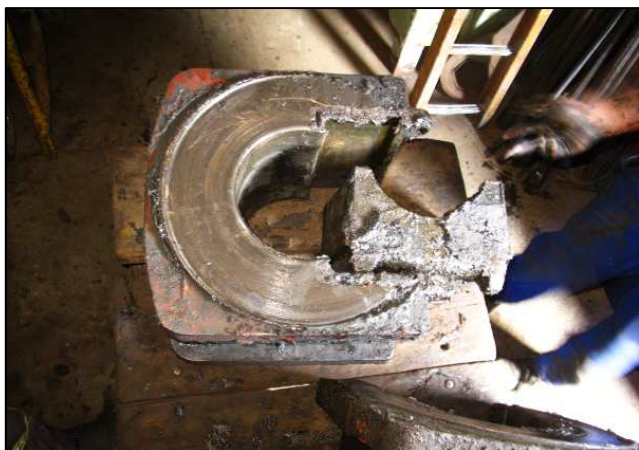
P07 - The axle bearings are worn at their crowns (left in the picture) which means the axles are not running true. The skew axles are imposing uneven wear on the thrust faces, and the small, but vital, driver axle side-play is reduced.
