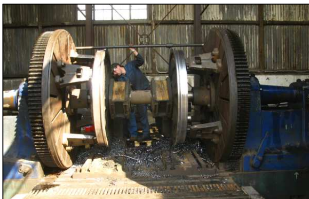
P10 - The fourth and final driver axle was being turned in the 1921 Craven wheel lathe for most of the day. The restored lathe is performing quite well both mechanically and electrically. The motor draws a steady 45 amps and the lathe doesn't strain on heavy loads.
