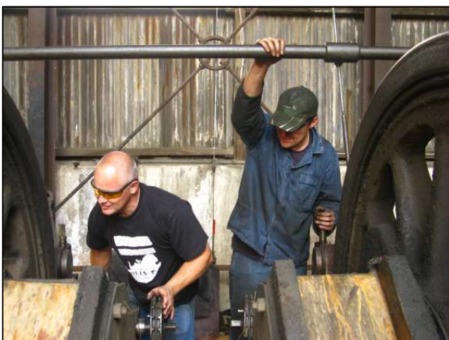
P11 - Dawie's pet fitter was here for the day too, a forlorn rescue picked up from the SATS Millsite Shops. Both gents are wearing safety goggles. We've found the lathe generally aims the spiral swarf towards the floor. But on the thicker cuts, you get the dangerous and unpredictable pings and chips that fly upwards towards the operator.
