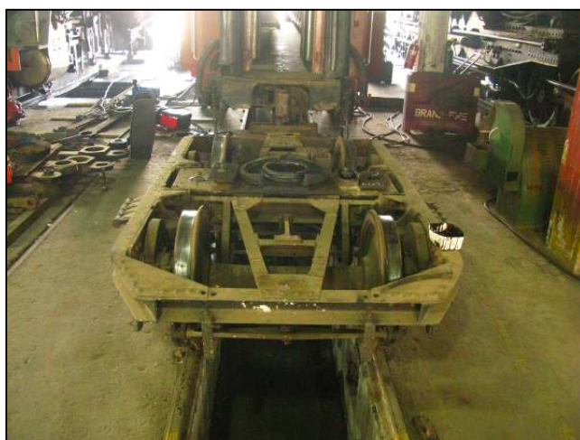
P24 - This coach needs axle work as there has been dragging damage to the wheel treads. So this isn't a one-day job. The wheel lathe CAN turn C&W axles but using two carrier dogs instead of four. (As per loco axles)
