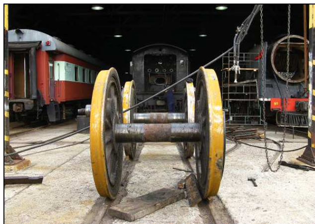
P08 - Just prior to putting a protective layer of grease onto the axle journals, the bare steel of the freshly-peeled wheels are already starting to rust with the morning dew-fall. (In the words of House Stark of Westoros, 'Winter is Coming.')
