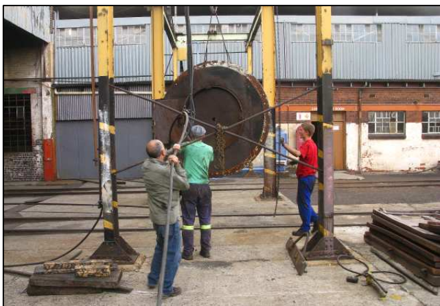
P19 - Traversing the smokebox front plate over that cruciform bracing was a tight squeeze and it JUST fitted. The plate needs to be descaled and repainted. We no longer use graphite paint, so this will be black etch primer,
