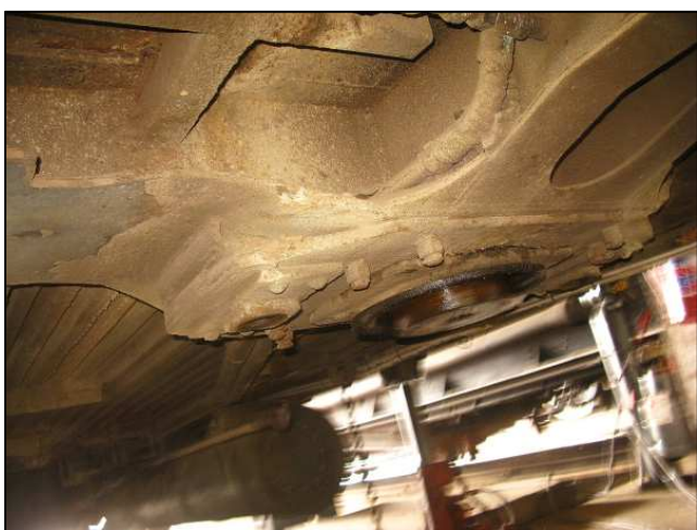
P23 - The bogie bolster pivot that has to be exposed and serviced at intervals. Notice the indented pads on either side, into which the sliding bearers of the previous picture engage.
