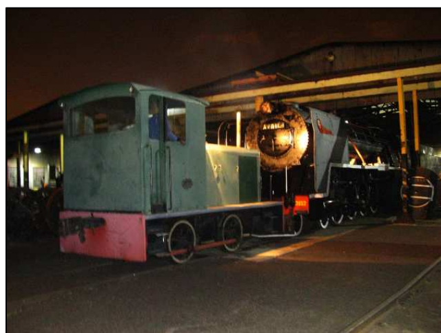
P24 - The last job of the day was to shunt the loco out so the chimney would be clear of the unventilated workshop roof. The safety valves also needed to be clear of the roof as they would be allowed to blow-off for calibration.
