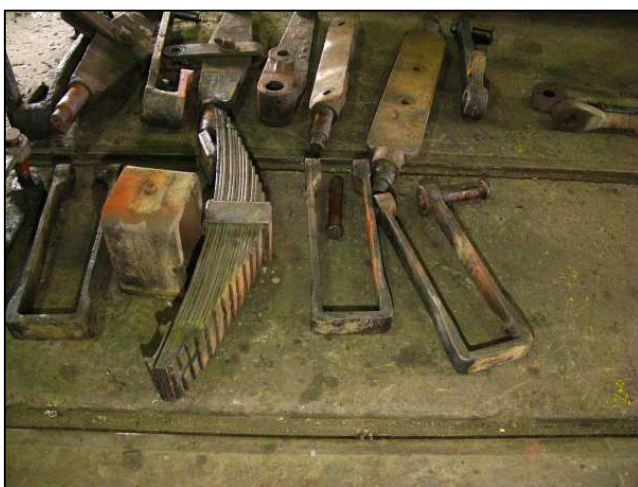
P27 - A growing collection of suspension and brake parts. All of them have been stamp-marked with their wheel allocation to be able to be returned from whence they came. Bushes may need to be custom fitted per component.
