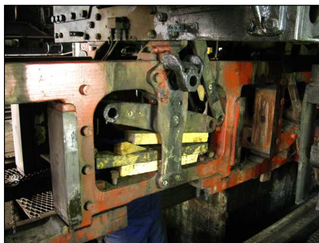
P28 - If time permits, greasing facilities will be added to the equaliser link pivots (center) and to the brake beam hangers. Due to their inaccessibility behind adjacent wheel rims, they are prone to not being lubricated on a regular basis, and have no engineered lubrication points anyway.
