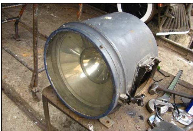
P15 - A closer view of the classic style Pyle National headlamp. This particular example is interesting as it has a retro-fitted GE sealed-beam unit in the middle, rather than the very obsolete Romania-made incandescent globe.
