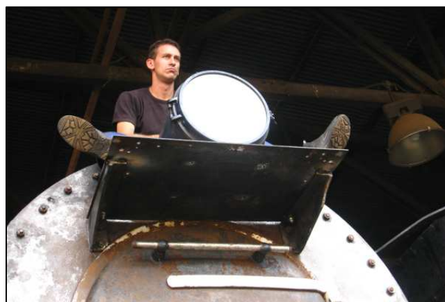
P16 - Test-fitting the 'new' headlamp. The name plate was later mounted on the forehead rail instead of from under the bracket (as is usual practice.) The problem with the easier bracket mount is that the name plate then has to be removed whenever the smokebox door is opened.
