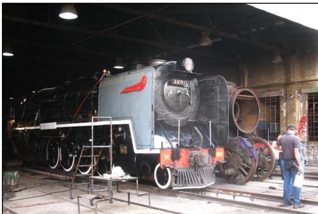
P03 - The first coat on the front end is done. She will be receiving a second coat of paint on the smokebox at a later date, while the cow-spreader and buffer beam would be painted by hand the following week.
