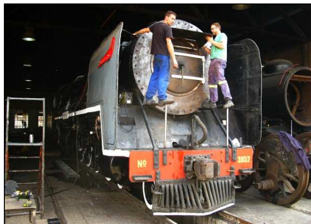
P14 - 15F 3052 was gifted a deeper headlamp bracket to accommodate a classic Pyle Chicago-style headlamp. As the smokebox front plate's mounting holes had been drilled skew in the past, it is rotated to the right slightly. The fellows dismantled the brackets and put shims on the right side to level the headlamp relative to ground level.
