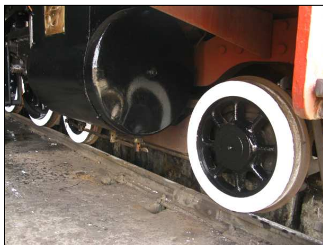
P06 - The cylinders were cleaned and the cylinder head covers were repainted as well. Interesting 15F fact. The cylinder bore and stroke (24 in x 28 in) matches that for the rebored 15CAs and the Class 23s as built.
