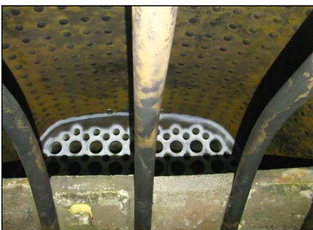
P11 - The firebox is done. The tube beads were welded during the previous week. If you look carefully, you'll see two of the fusible plugs screwed into the crown sheet at the front center.
