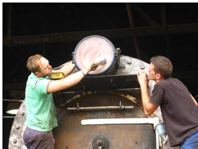
P18 - Painting the headlamp glass with grease to protect it from paint gun over-spray. The paint overspray then comes off with a paraffin rag. This is much easier than using masking paper on a circular surface!
