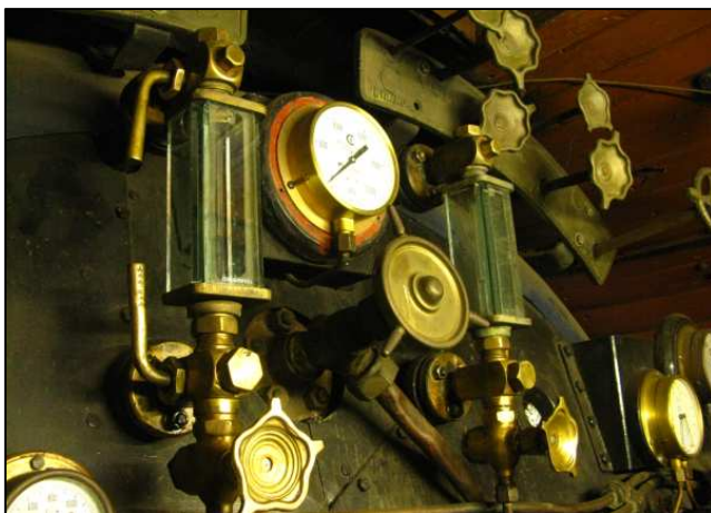
P13 - The cab is coming back together. Both the main pressure gauge and the duplex vacuum gauges were SANAS calibrated and certified. The turret spindles and their universal joints still need some work. We plan to move the speedometer a few inches to the left, as it is obstructed by the brake ejector's steam pipe.
