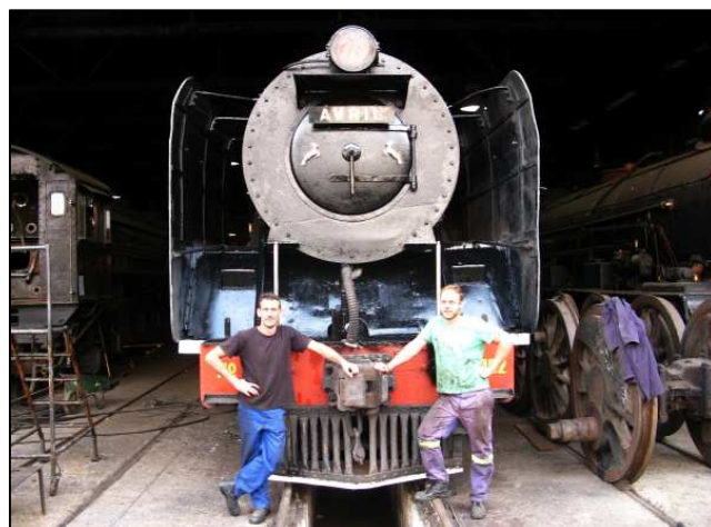
P04 - The newly reassembled front end at the end of the work day, with all of the external fixtures bolted back on. Just missing a nose wheel, which was left off in case access was needed to the smokebox on test day.
