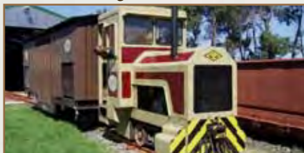
Funkey Shunting underground Mine locomotive converted by Sandstone for above ground use.
