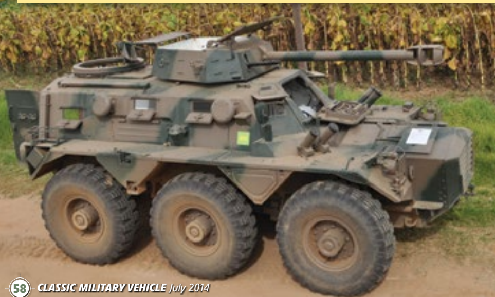
Above: The Eland 60mm mortar originated from the French Panhard but had a 2.5-litre Chevrolet engine and was assembled in South Africa during the Bush War. It formed the mainstay of South African armoured units.
